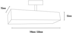
CODE WATTAGE **BOARD OUTPUT** LAMP TYPE DIMENSIONS **DIMMING OPTIONS** LYF13 1280lm 8W 3000k LED 190mm x 93mm x 55mm Phase cut (leading/trailing edge) LYF14 8W 1340lm 4000k LED 190mm x 93mm x 55mm Phase cut (leading/trailing edge) LYF33 3000k LED 320mm x 93mm x 55mm Phase cut / DALI 16W 2560lm LYF34 16W 2680lm 4000k LED 320mm x 93mm x 55mm Phase cut / DALI
