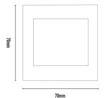
CODEWATTAGELAMP TYPEDIMENSIONSLEDSTLGL2.2W3K LED 200 lumens70mm x 70mm - 65mm x 65mm cut out
